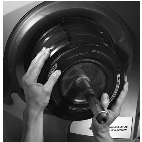
Step 2: While pressing pack towards machine, turn counterclockwise about 10 degrees until all six plate tabs lock into place. Then turn clockwise until index marks are aligned.
